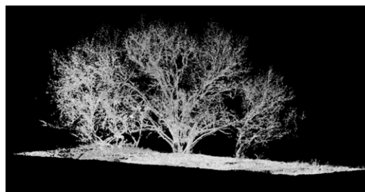
FIGURE 3.11 (See color insert following page 426.) Ground-based lidar data collected over Mesquite trees in central Texas.
