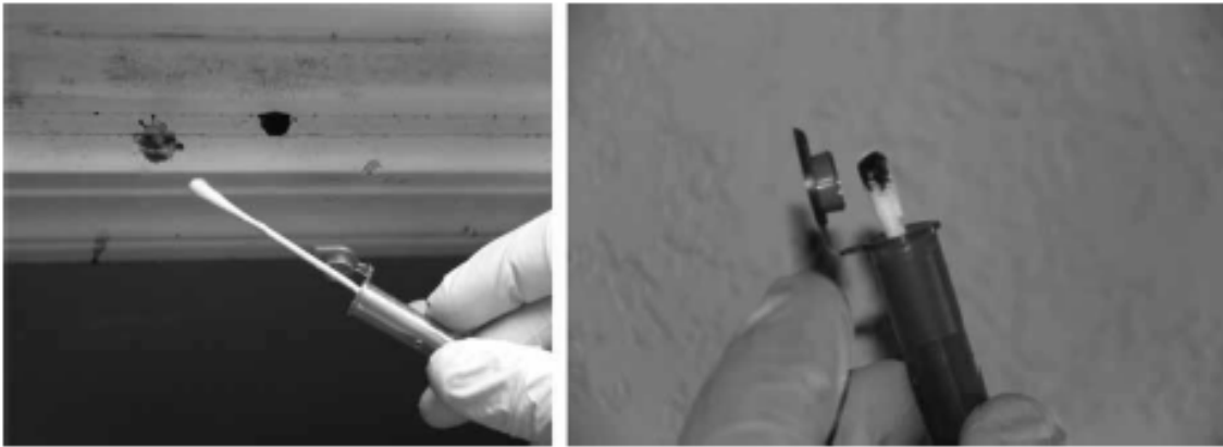
Figure 41.5 Collection of a wet sample of blood using a swab fitted with integrated swab cover to allow for drying and prevent contamination.
