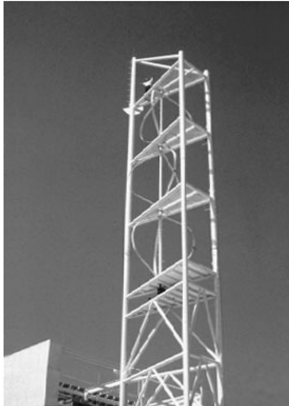
FIGURE 9.4 Three stacked wind turbine (Darrieus), 4 kW each, next to building. Notice man on top. (Photo courtesy of Coy Harris, American Wind Power Center and Museum.)
