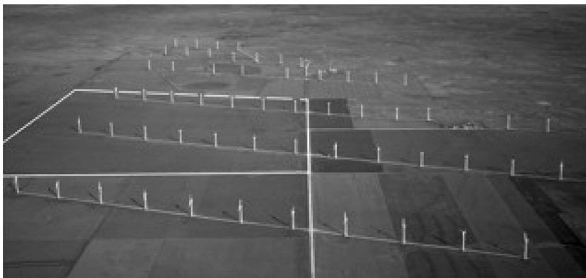
FIGURE 9.11 West side of wind farm in plains near White Deer, Texas. White lines are roads, to show one square mile, which is equal to 260 ha. (Photo courtesy of Cielo Wind Power.)
