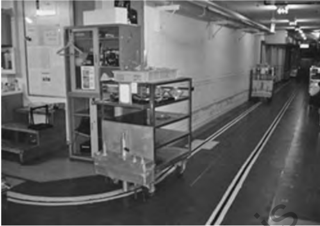
FIGURE 3.2 Kaga Shop food automated transport system.
